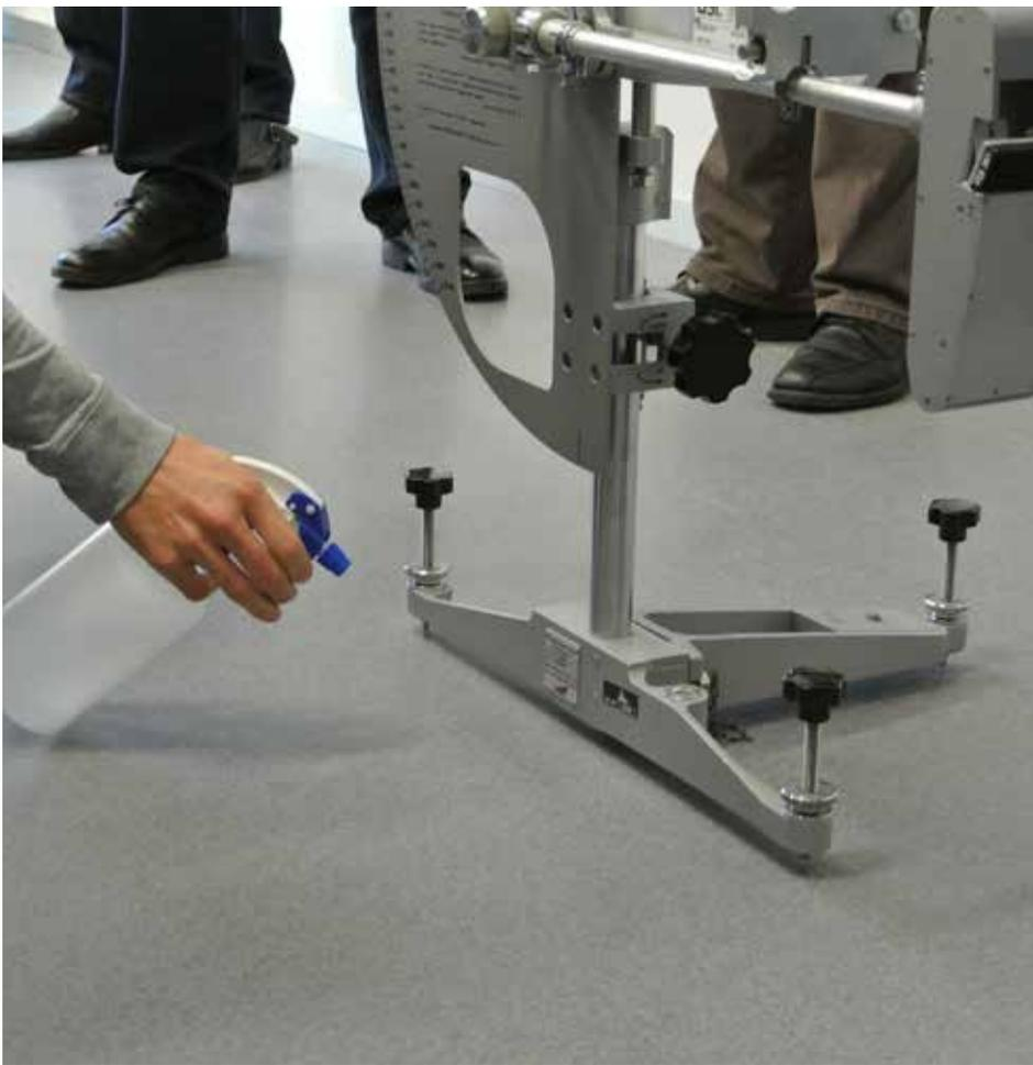
Figura 1: TRRL Pendulum Tester.
